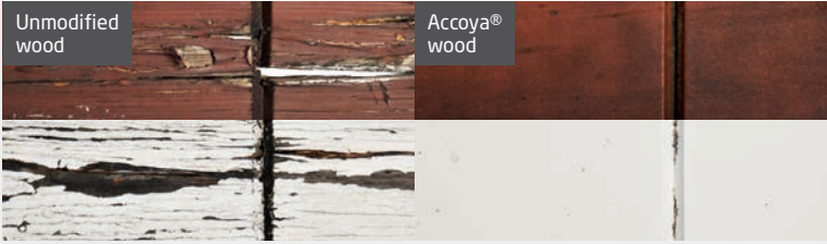
Coating comparison after 13 years outdoor exposure
